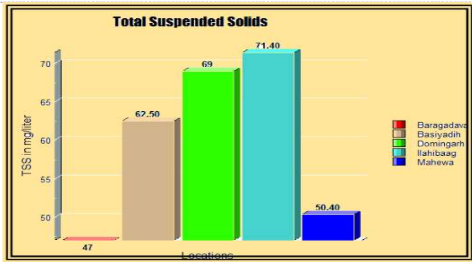
Fig4: Total Suspended Solids(TSS) for Selected City Sewers
